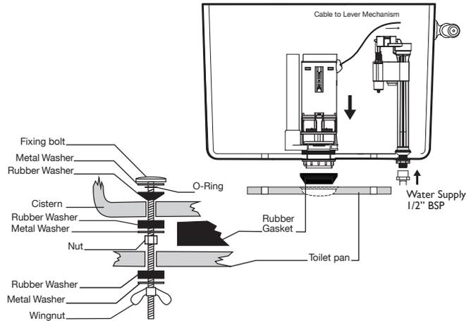
Mount the cistern to the WC pan as shown above. Ensure the gasket is firmly sealed around the flush channel. Once assembled the toilet can be positioned and installed in location. Before securing the pan to the floor, drill the holes in the wall for securing the cistern tank. After securing the pan to the floor, attach the tank to the wall using fixings suitable for the installation in hand (not supplied).
