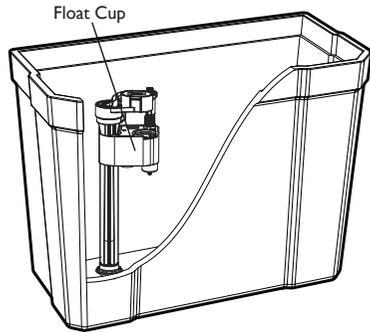
The fill valve is supplied set at a height suitable for the cistern tank. Please ensure that all connections are fully tightened before progressing.
