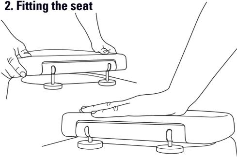
Align and insert the pins into the seat hinge sockets and firmly press down until you hear them 'click' into position. Adjust the hinge anchors to make sure the seat lines up with the edges of the toilet pan. When you are satisfied the seat is in the correct position, remove the seat from the hinge anchors (see step 3) and fully tighten the screw in the Top Fix Insert (shown in step 1). Place the Cover Plates over the Hinge Anchors. Replace the seat and click into position.
