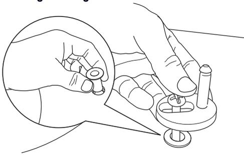
Place the Top Fix Inserts into the fixing holes in the toilet pan. Insert the screws within the Hinge Anchors as shown and begin to tighten the screws until they are loosely secured, to allow for adjustment of the seat on the pan.
