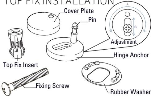
Maximum adjustment of the pin position is achieved by rotating the hinge anchor around the screw (adjustment A in the parts diagram above). Further fine adjustment of the pin position can be achieved by sliding the screw in the adjustment plate (adjustment B).
