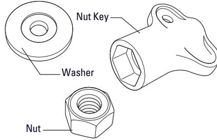
To be used with Fixing Screw, Hinge Anchor, Rubber Washer & Cover Plate if the top fix kit is unsuitable for installation.
