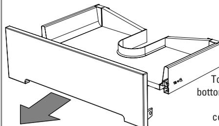
To return the fascia, locate the bottom fixings into the sides of the drawer and re-fix the plastic covers. Re-fix the rails on both sides of the lower drawer.
