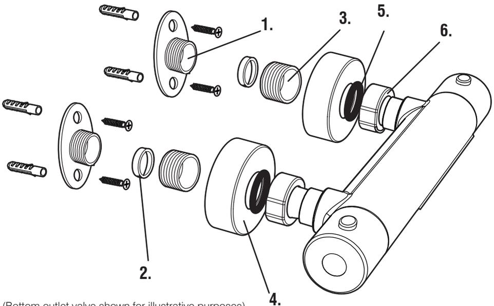
1. Install hot and cold inlet pipework (15mm) to the desired installation location - ensuring the pipes are 150mm apart and protude at least 35mm from the finished wall surface.
