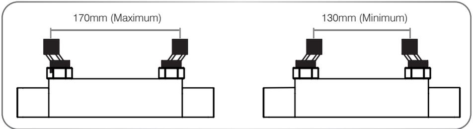
1. Install hot and cold inlet pipework (15mm) to the desired installation location. Standard bar valve centres are 150mm apart.
